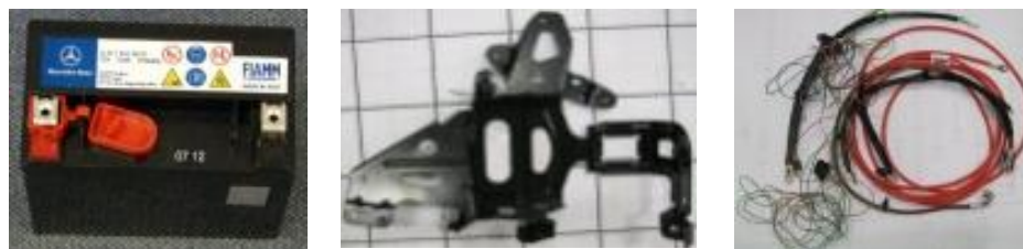
Figure D-47: New Technology Battery, Mounting Bracket & Harness
