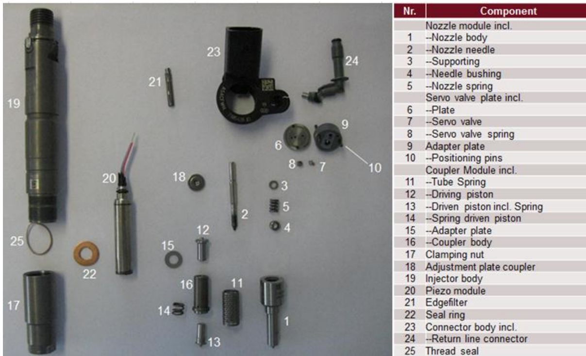
Figure B-3: Initial Level of Injector Teardown
